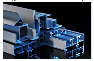
uPVC and aluminium that have been preshaped to Shinyglas' requirements by their manufacturers using a process called "extrusion". The resulting extrusions are supplied as long lengths of uPVC or aluminium. Shinyglas makes frames by cutting sections of extrusion to their required lengths before joining them together with the appropriate brackets and hinges.
